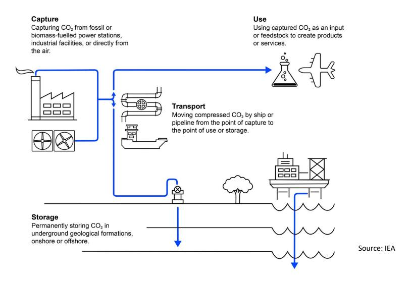
Carbon Capture provides an immediate solution for decarbonisation
